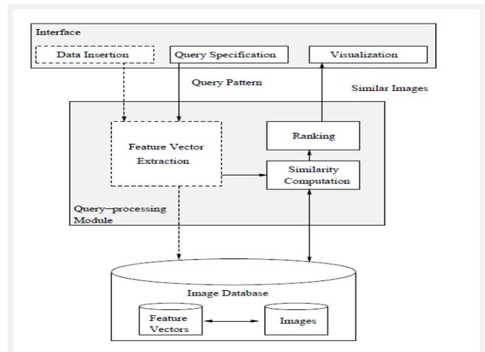
Fig. 2 Typical Architecture Of Content Based Image Retrieval System[2]
